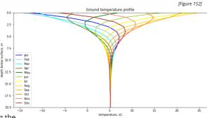
In January, when the air temperature is close to -15 degrees, the ground temperature at just 3m below ground is 7 degrees. This coupled with solar gains during the day makes for a very effective ground source heat pump.
