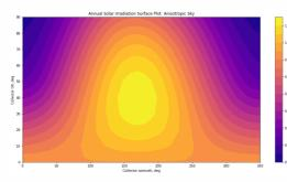
PV solar panel collector : (Y) angle and (X) orientation
