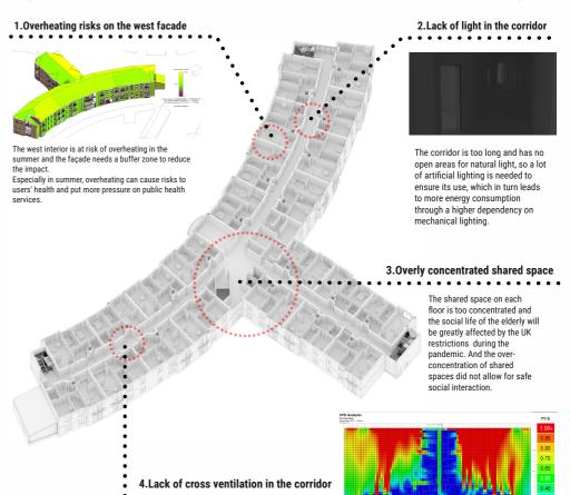
The lack of open spaces makes cross ventilation in corridors ineffective. As recommended in A03 and A06 of the WELL standard, enhanced ventilation strategies can help dilute human and product generated air pollutants and reduce indoor C02 levels. As mentioned on page 7.9, occupants are used to opening the doors of their rooms for ventilation in summer. During the current pandemic, it was not possible for residents to cross-ventilate by opening communal/corridor doors and windows
