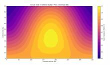
PV solar panel collector: (Y) angle and (X) orientation
