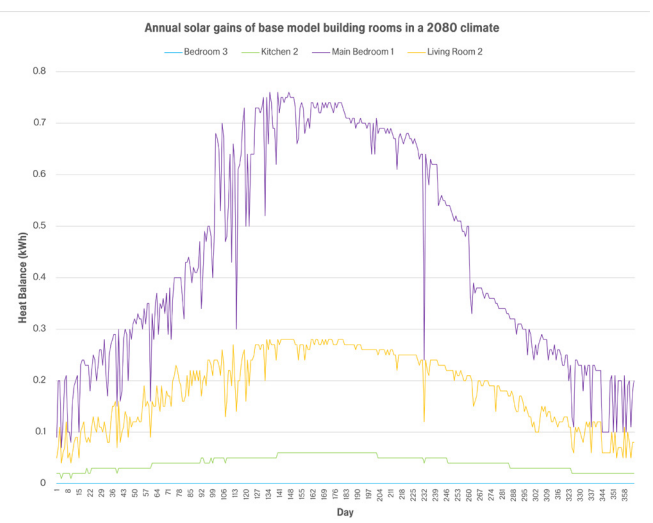
Figure 6.8: [left] The solar gains in a current climate. [right] The solar gains in a 2080 climate. It is optimal if the lines on the chart stay as low on the Y axis in the summer months to avoid unwanted solar gain. Therefore bedroom 3 performs the best and main bedroom 1 performs the worst.
